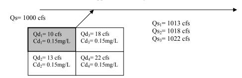
Note: Qs is the **7Q10** stream flow.  $Qs_1$ ,  $Qs_2$ , and  $Qs_3$  are the stream flows (i.e., **7Q10** plus facility flow) downstream of the WWTF after the first, second, and third expansions, respectively.
