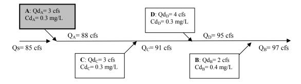
Note: Qs is the **7Q10** stream flow.  $Q_A$ ,  $Q_B$ ,  $Q_C$  and  $Q_D$  are the stream flows downstream of Plants A, B, C, and D respectively (i.e., **7Q10** plus facility flows).
