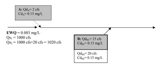
Note:  $Qs_1$  is the flow upstream of the affected **segment** (i.e., upstream of Plant A) and  $Qs_2$  is the flow downstream of Plant B after the consolidation/expansion.
