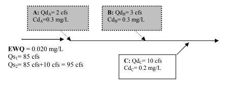
Note:  $Qs_1$  is the flow upstream of the affected **segment** (i.e., upstream of Plant A) and  $Qs_2$  is the flow downstream of Plant C after the consolidation.
