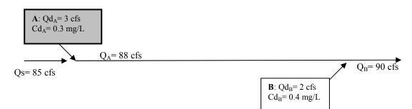
Note: Qs is the **7Q10** stream flow.  $Q_A$  and  $Q_B$  are the stream flows downstream of Plants A and B, respectively (i.e., **7Q10** plus facility flows).
