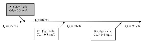
Note: Qs is the **7Q10** stream flow.  $Q_A$ ,  $Q_B$ , and  $Q_C$  are the stream flows downstream of Plants A, B, and C, respectively (i.e., **7Q10** plus facility flows).
